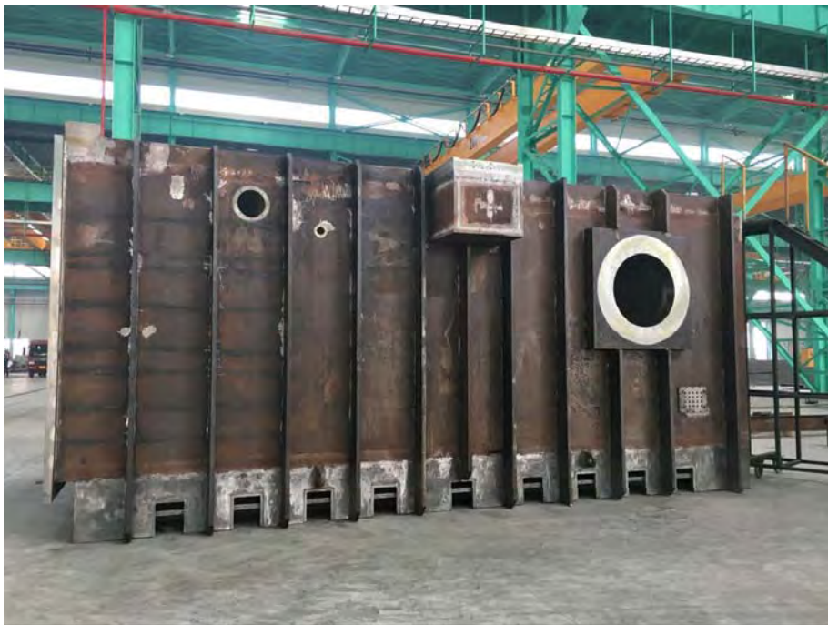
Vacuum Chamber Q235B+304 Cladding Material
